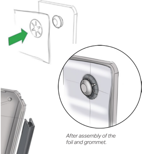
Figure 6e. EMI shielding foil held in place by formed metal standoffs around the grommet, requiring no adhesives.
