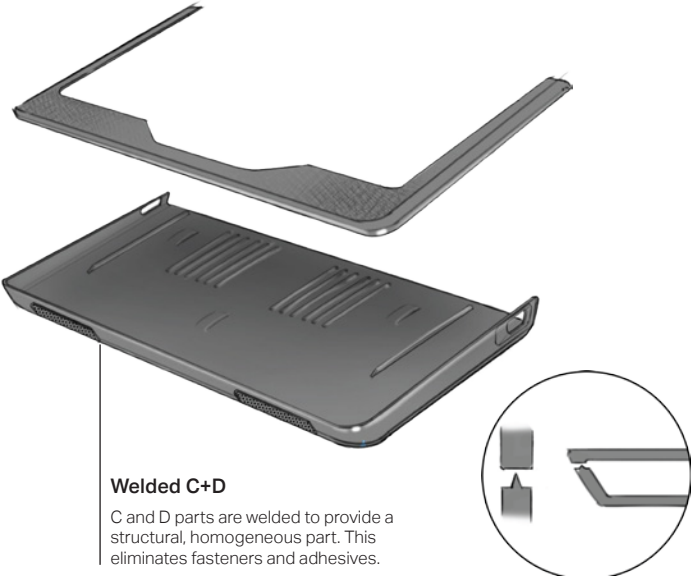
Cross-section shown before ultrasonic welding.
